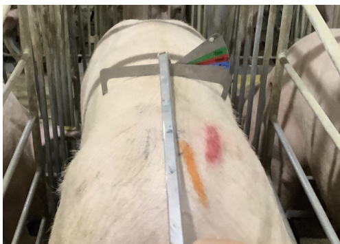
The above image displays a sow caliper. Sow caliper’s are used to gather an objective measurement on sow body condition score.
